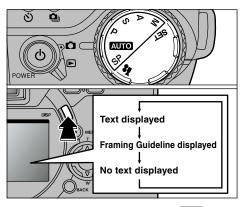
This function can be selected in the "AUTO  $\cdot$  SP  $\cdot$  P  $\cdot$  S  $\cdot$  A and M" photography modes. The screen display changes each time you press the "DISP" button. Press the "DISP" button to display the framing guideline.
